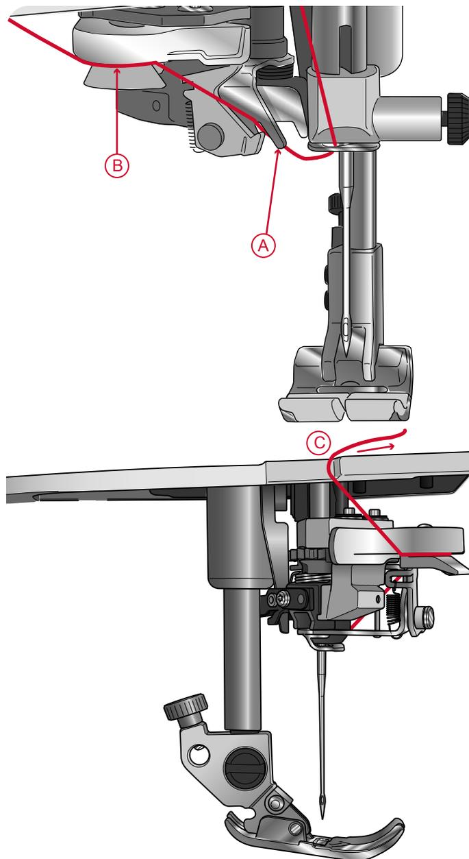
3. Touch the automatic needle threader button. The presser foot is automatically lowered during the threading sequence, and will rise again when threading is finished.
