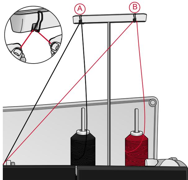
*Note: When using large thread cones on the auxiliary spool pin, place the large spool holder with the flat side up and a cone holder on the spool pin before adding the thread cone.*
