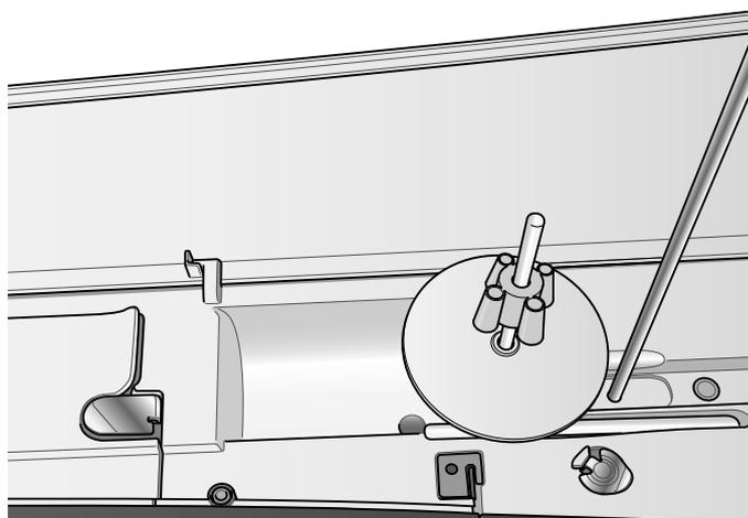
3. Hold the thread with two hands as illustrated. Floss the thread under the thread guide (A) from front to back. Pull thread back into and through threading slot (B).
