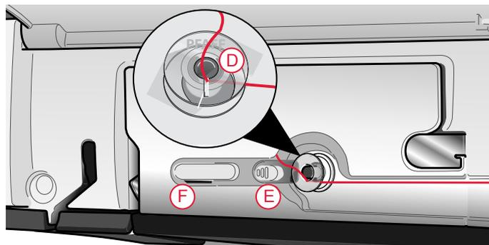
4. Push the bobbin winding lever (E) towards the bobbin. A pop-up appears on screen. To adjust winding speed drag the slider. Hold the thread end firmly when starting to wind. Touch the play button in the popup window and let the thread wind a few turns. Touch the pause icon and cut the loose thread end close to the bobbin. Press play again.
