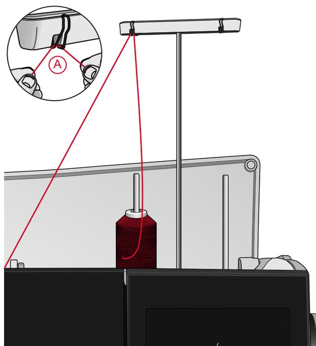
*Note: When using thread cones, place a cone holder on the spool pin before placing the thread cone. This prevents the thread cone from wobbling.*
