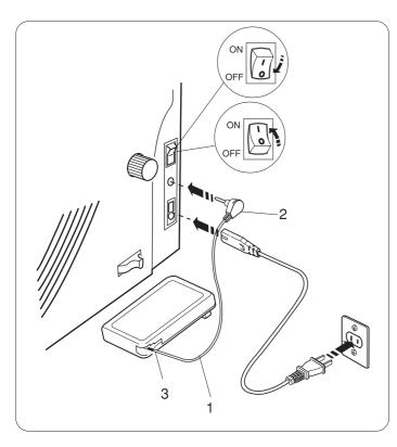
If you wish to use the foot control, pull out the cord from the foot control and insert the pin connector into the jack on the machine.
