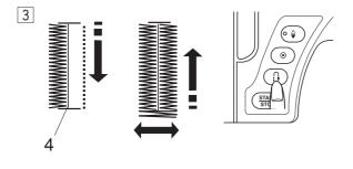
3 Start the machine again. The machine will sew back to the starting point then will sew the front bartack and right row.
