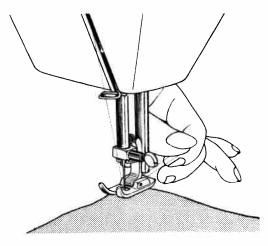
Fold edge of material. With folded edge to left, place it under presser foot.
