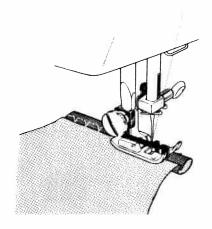
Sew carefully, guiding fold against guide so that straight stitches are made on hem edge, and slanting stitches pierce only one or two threads of fold.
