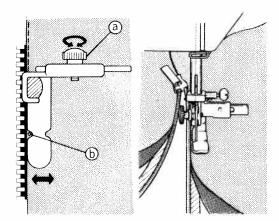
Loosen screw (a) and set foot so that needle comes into position (b). Tighten screw.
