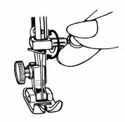
With flat face away from you, insert a new needle into groove of needle bar.
