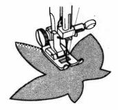
To change direction at corners, or to sew very small circles, stop machine, positioning needle just away from edge of cut-out, lift presser foot and turn material. Lower presser foot and continue sewing.
