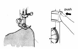
Release button and commence forward sewing guiding fabric by hand as it is fed. Never pull material.
