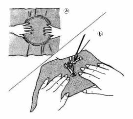
Stretch fabric over the hoop ⓐ or sew with free arm ⓑ according to the part you are going to darn.
