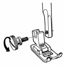
Remove foot by loosening screw with screwdriver.
