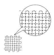
Sew over the worn-out part with closely spaced, stiches guiding material back and forth by hand.
