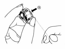
Pulling thread to left, bring it under tension spring then to delivery eye **(b)**.
