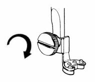
Replace new foot and tighten screw.
