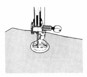
Position a button and material under foot. When needle comes to left side of stitch, lower foot. Raise needle and adjust zigzag width so that needle comes to right hole of button.
