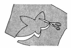
Sew around outline with zigzag stitch adjusting stitch length and width according to shape and size of cut-out and type of base material.
