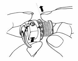
Guide thread into slot (a) of bobbin case.
