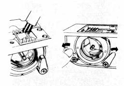
Remove hook race cover. Remove hook. Clean hook race with a cleaning brush and a soft cloth.
