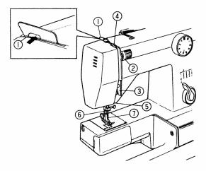
Lead thread either side of tension disc ②.
