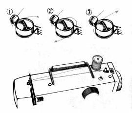
Wind thread clockwise around bobbin several times. Push bobbin on to spindle.
